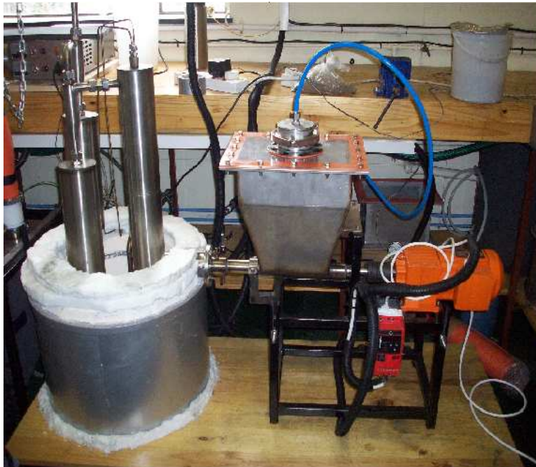
Figure 59: Picture of cyclones (C05 & 06), reactor (R04) and feeding system (F02), (from left to right).
