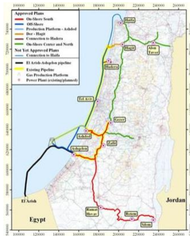
Figure 2.4: Natural gas transmission system
