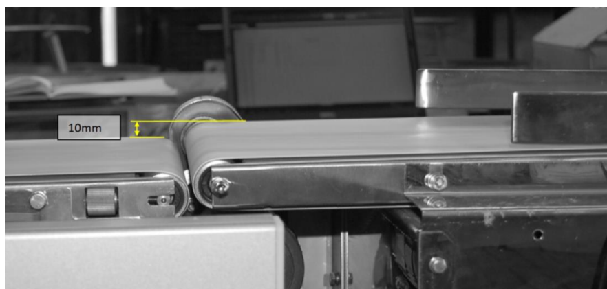
Figure 6.26: Height level difference between load cell and separator conveyor belts
