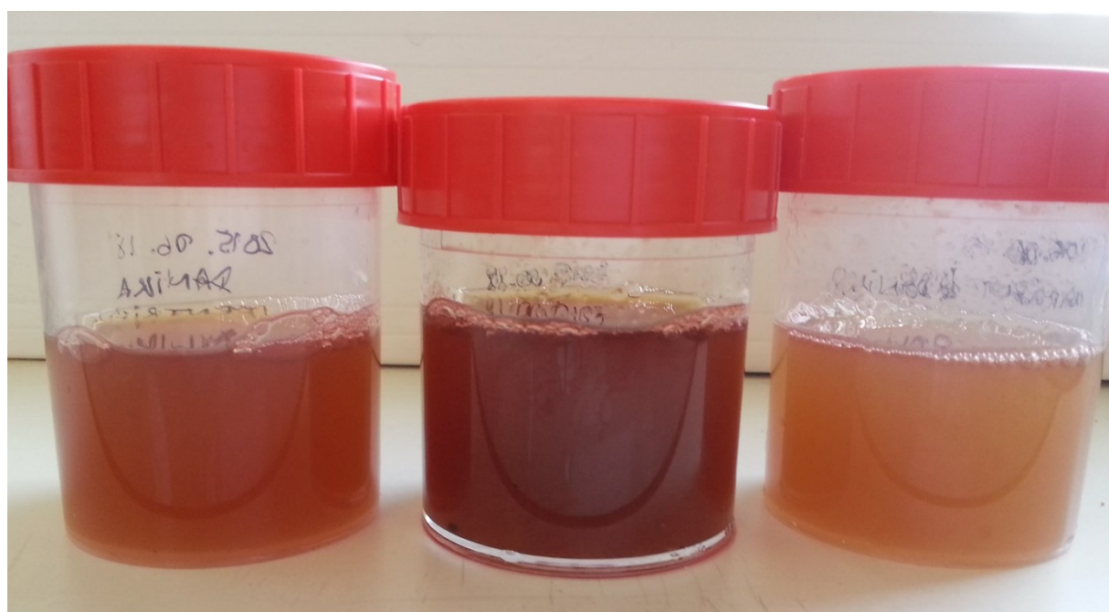
Figure 3.9 Liquid fractions obtained after alkaline extraction of AX from wheat bran on large scale and centrifugation (left), ultrafiltration (centre) and chromatographic discolouration (right).
