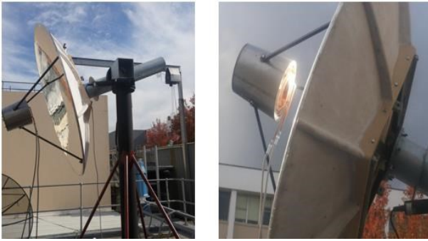
Fig. 7 Parabolic dish and conical receiver set up.
