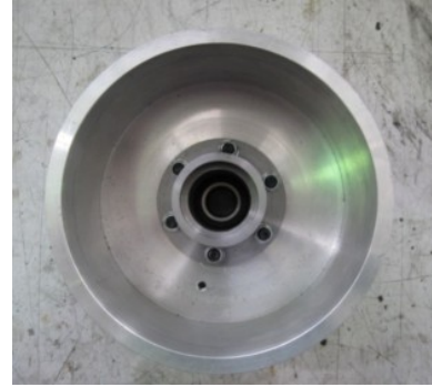
Fig. 3.2 Small prototype solid aluminium slip rotor.
