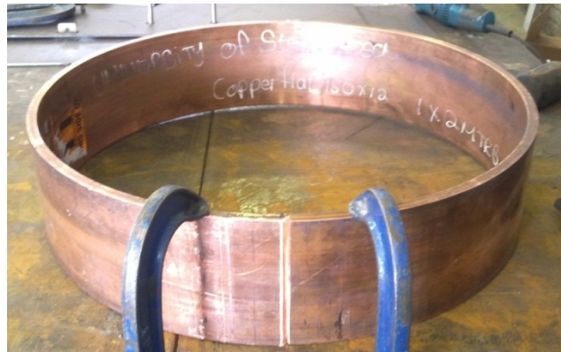
Fig. 4.13 Rolled copper ring during slip rotor manufacture process.
