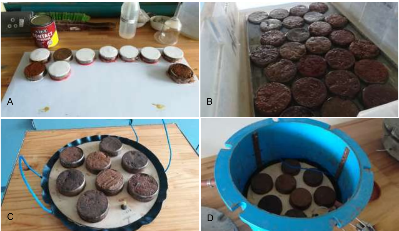
Figure 4.1: Filter papers were glued at one side of the cores to ensure good contact between the cores and pressure plates (A), thereafter, the cores and the pressure plates were saturated in a water bath (B). The saturated cores were transferred on the pressure plates (C) and were inserted in a pressure chamber which ran for two to 16 days until the equilibrium was reached (D).
