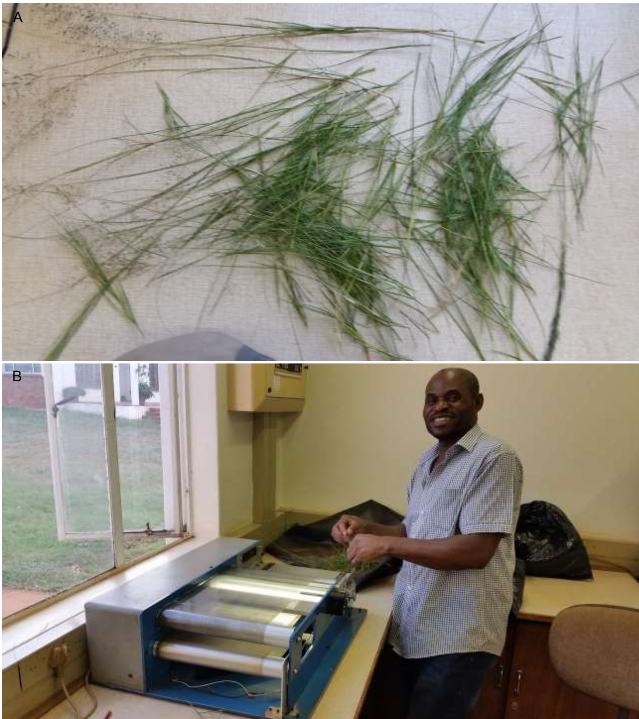
Figure 5.2: Relative low photosynthetic active leaf area for grasses as the leaves are narrow (A) and the LI-3100C Area Meter used to determine the leaf area index (B).
