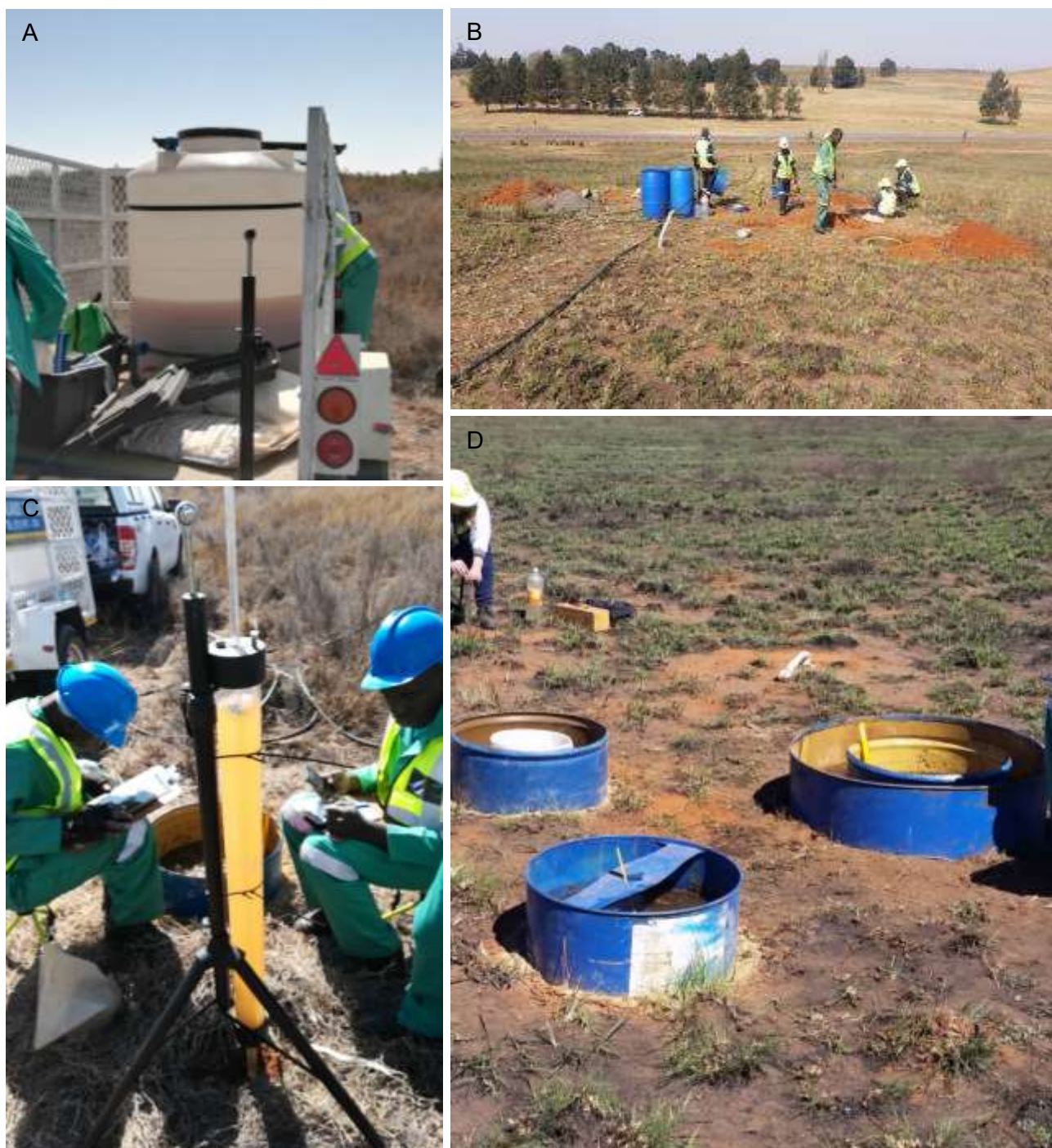
Figure 3.1: The water tank used to store water for infiltrometer tests (A) and conducting infiltrometer tests and excavate test pit (B). Pipe and drum system was used to provide water at Discard Dump 1 & 2. The infiltrometer tests were conducted with a constant-head permeameter (C) and in the picture at the bottom right-hand side (D), single-ring infiltrometer in front, large double-ring ring infiltrometer at right and standard double-ring infiltrometer at left were also used for infiltrometer tests.
