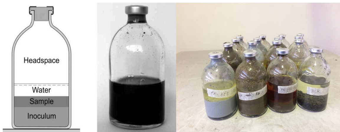
Figure 3-3: Biomethane potential test (schematic diagram obtained from Angelidaki et al , 2009)
