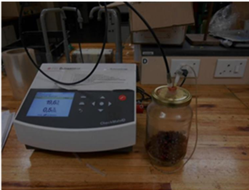
Figure 2. Gas sampling using Checkmate 3, PBI Dansensor gas analyser.
