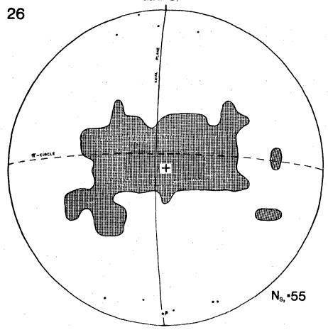
Compilation of subfabrics ( $S_2$ -poles and mesoscopic fold axes), domain 1 (Map 3, De Trap). Contour at 0%.
