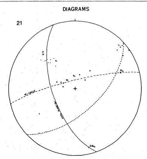
Stereographic compilation of  $S_1$ ,  $S_2$  and  $L_1$  of an anticline in the lower part of the Fold Zone(De Trap).
