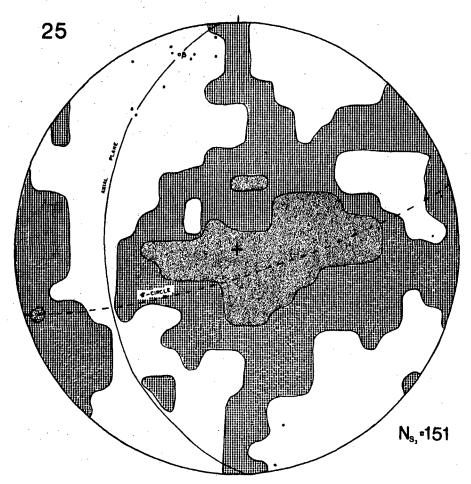
Compilation of subfabrics (S3-poles, mesoscopic fold axes and L2), domain 2 (Map 3, De Trap). Contours at 0% and 3%.
