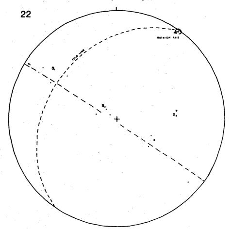
Stereographic representation of the transposition of S1 to S3 (De Trap).
