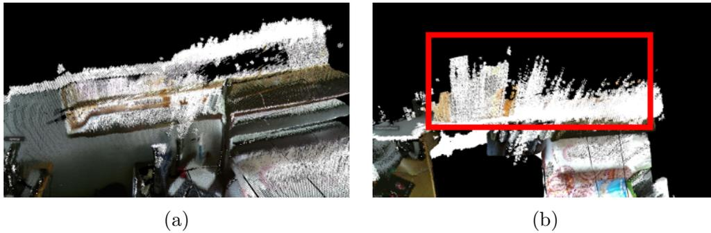
Figure 7.39: These figures illustrate the noisy points generated in the Room Closed Loop data set in the region of the window from two different angles. The spray of white points behind the surface is the noise generated from external factors.
