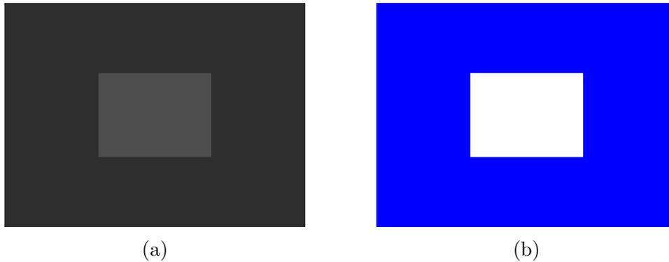
Figure 7.23: Test data that is used to illustrate the different point cloud extraction techniques. Subfigure (a) is the depth map that shows a depth measurement of 1 meter in the outer rectangle of the image and a 2 meter measurement for the inner rectangle. Subfigure (b) illustrates the associated RGB image that uses blue to represent the area that is 1 meter away from the sensor and white to show the area that is 2 meters away from the sensor.
