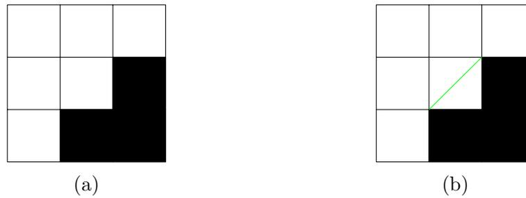
Figure 3.3: This figure demonstrates a configuration that requires the marching cube intersection method of generating a line in 2D. If this were in 3D, it would generate a triangle. White indicates the square is outside the model and black indicates the square is inside the model. The green line indicates the generated edge in the 2D case.
