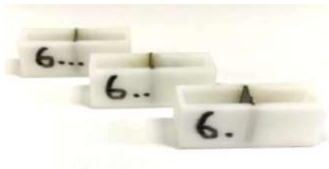
**Figure 5-11: Custom 3D-printed diffusion wells for vancomycin release screening of parameter set 6**
