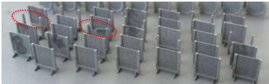
**Figure 7-1: As-built PTWs within support frame on build plate**
