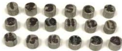
**Figure 5-3: Cylindrical specimens for porosity measurement**
