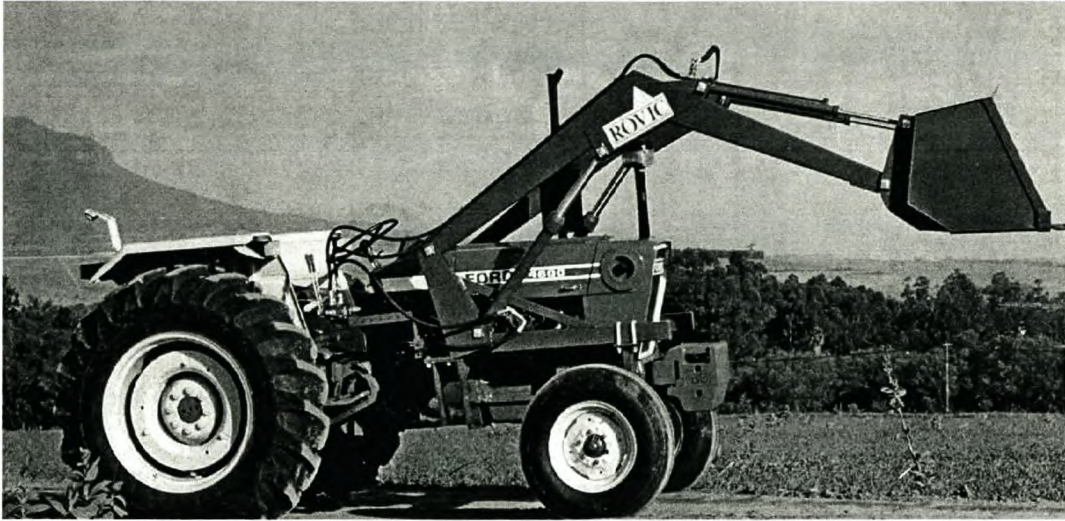
Figure 6 Typical example of a front-end loader fitted on a tractor with a kit
