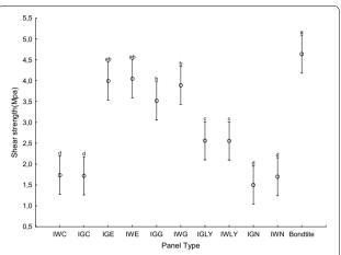
**Fig. 8** Shear strengths of Irvingia-based wood adhesives (Error bars with same or similar letters are not significantly different, p < 0.05)
