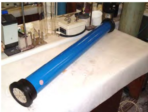
Figure 2: Side view of module for housing capillary membranes
