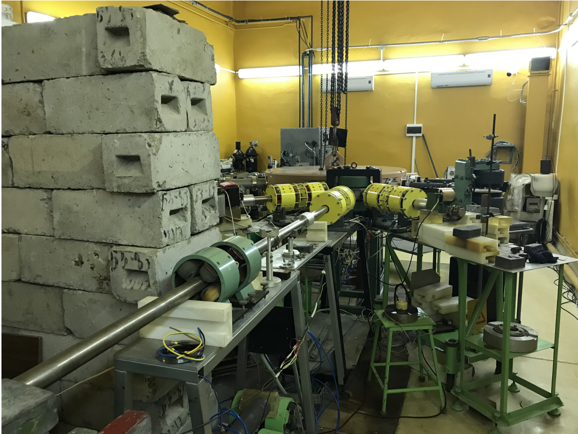
Figure 3.16: Picture of the VEGA experimental setup, the elongated flight tube of the can be seen extending from the center to the bottom left of the picture.
