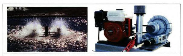
Figure 5.4 Paddlewheel aerator in action and backup blower
