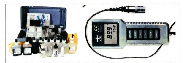
Figure 5.5 A basic water quality test kit designed for freshwater aquaculture by HACH, and handheld dissolved oxygen meter by YSI
