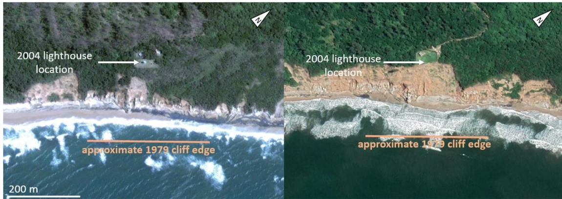
Figure 4.39 Satellite images comparing the erosion near the Richards Bay Lighthouse from 1979 (orange line), 2004 (left), and 2021 (right) (Google Earth, 2004b, 2021b; Sailing, 2018)
