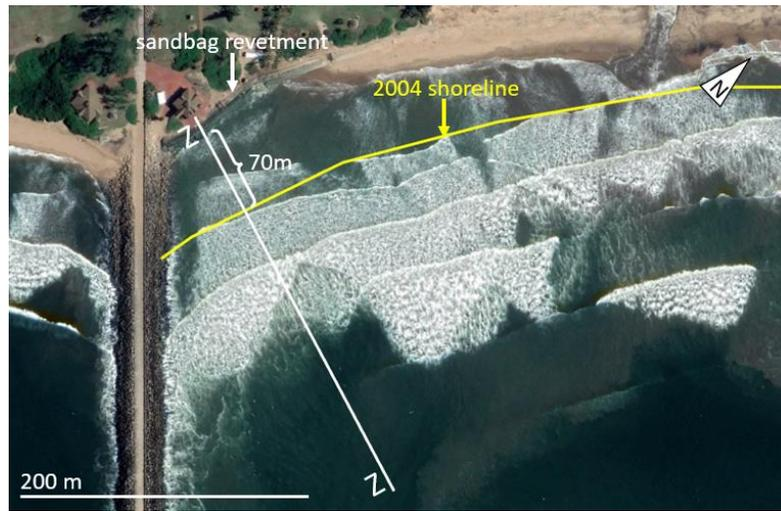
Figure 4.42 Cross-section Z-Z used to estimate a capital nourishment project with the 2004 shoreline 70 m seawards from the present (Google Earth, 2004b, 2022f)
