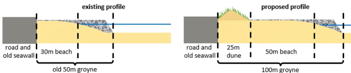
Figure 4.32 Reprofiling Ponta Gea beach at cross-section Y-Y (existing profile left and proposed profile right)
