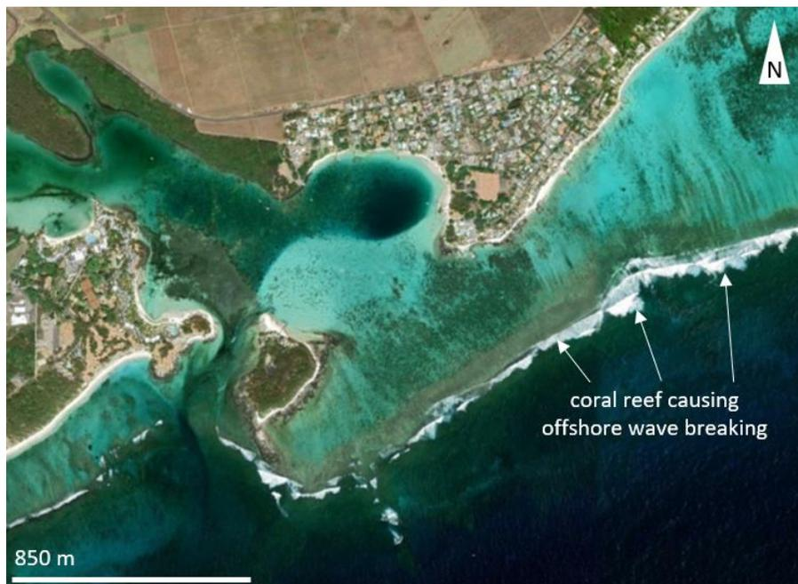
Figure 3.8 Fringing coral reef in Blue Bay Marine Park, Mauritius that causes waves to break offshore protecting the shoreline (Google Earth, 2022a)
