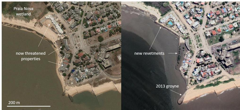
Figure 4.25 2012 and 2022 Satellite images of Ponta Gea beach comparing erosion west of groyne built in 2013 (Google Earth, 2012, 2022e)
