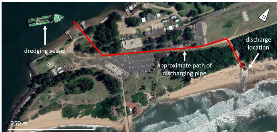
Figure 4.34 Satellite image capturing the dredging process at Alkantstrand, Richards Bay (Google Earth, 2022f)
