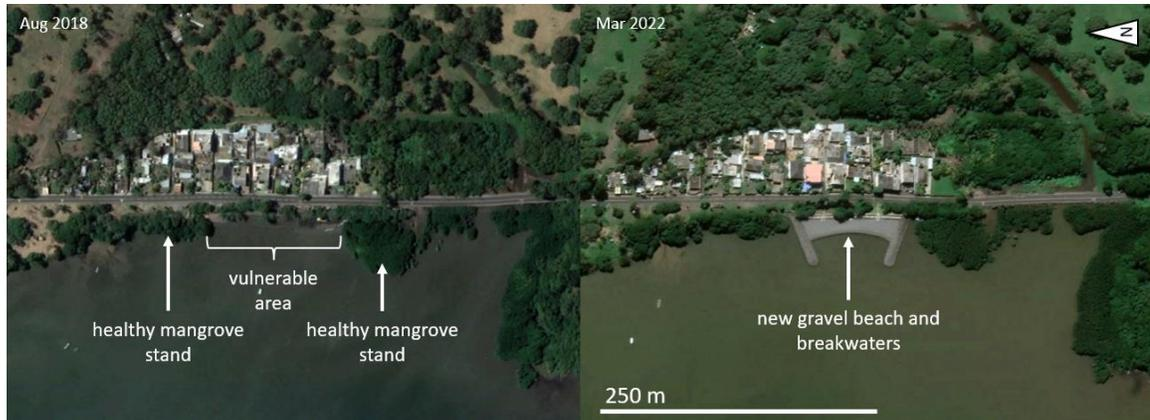
*Figure 4.6 Satellite Images of Case Noyale between August 2018 (left) and March 2022 (right)*
