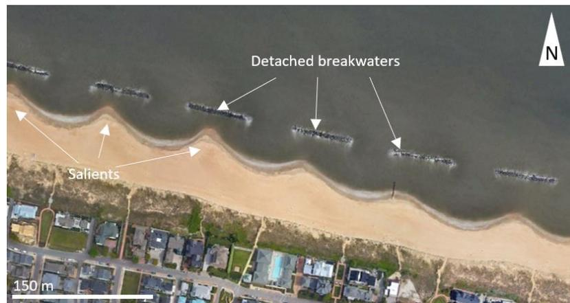
Figure 3.10 Detached breakwater at Norfolk Beach (Virginia, US) with salients forming leeward of the breakwater (Google Earth, 2019)
