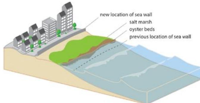
*Figure 3.19 Hybrid defence with seawall, salt marsh, and oyster beds (Sutton-Grier, Wowk & Bamford, 2015)*
