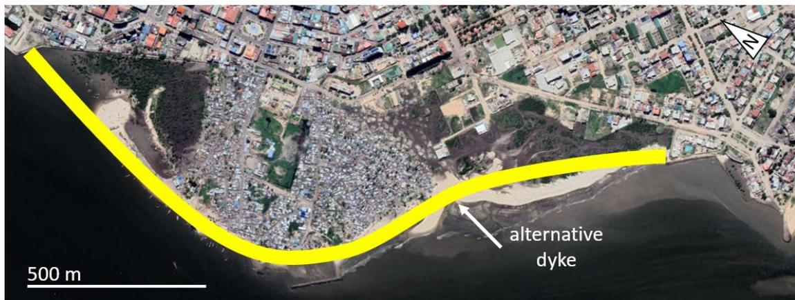
Figure 4.29 Alternative revetment or dyke option for Praia Nova (Google Earth, 2022e)
