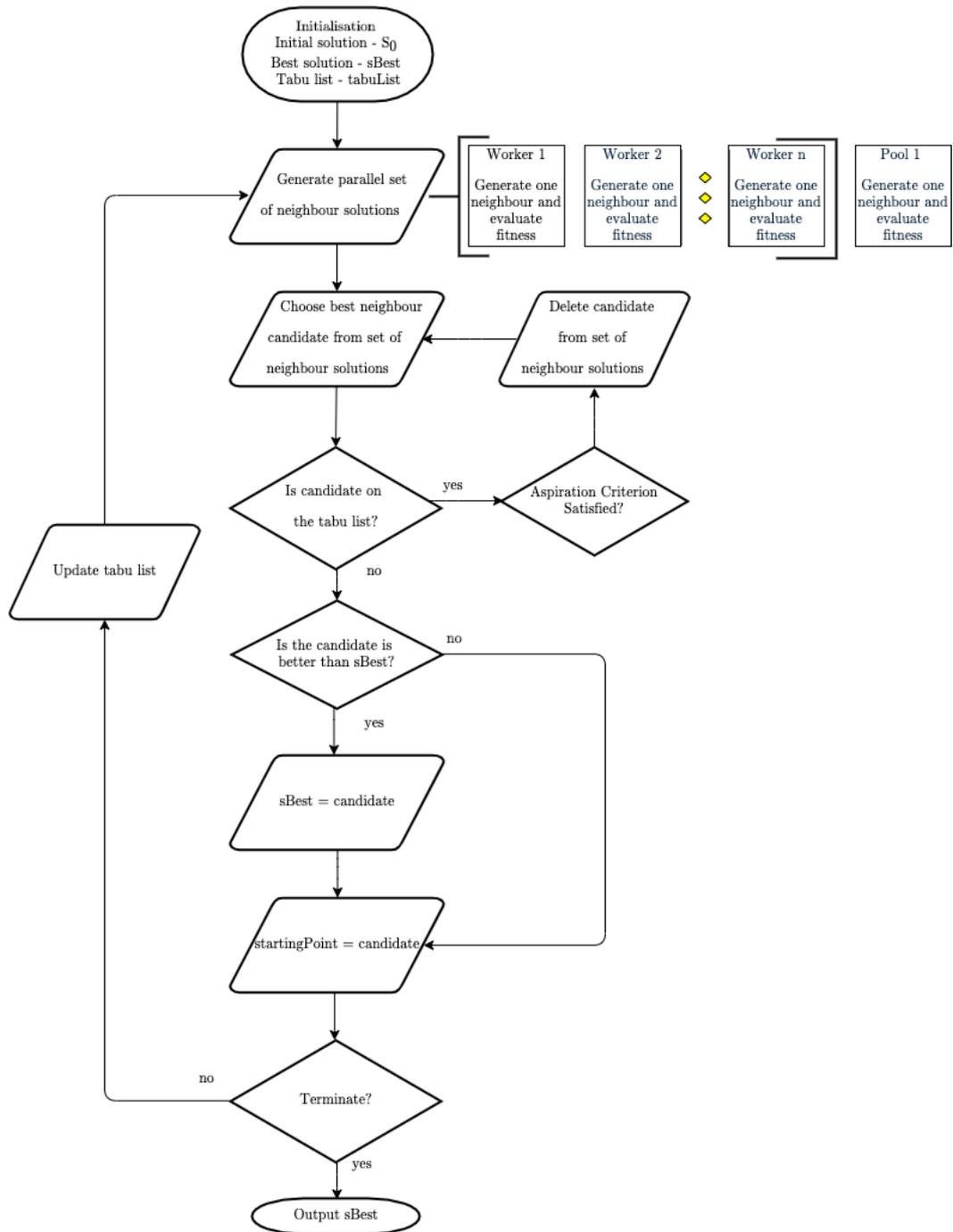
Figure 4.9: Tabu search (TS) with iteration-level parallel execution
