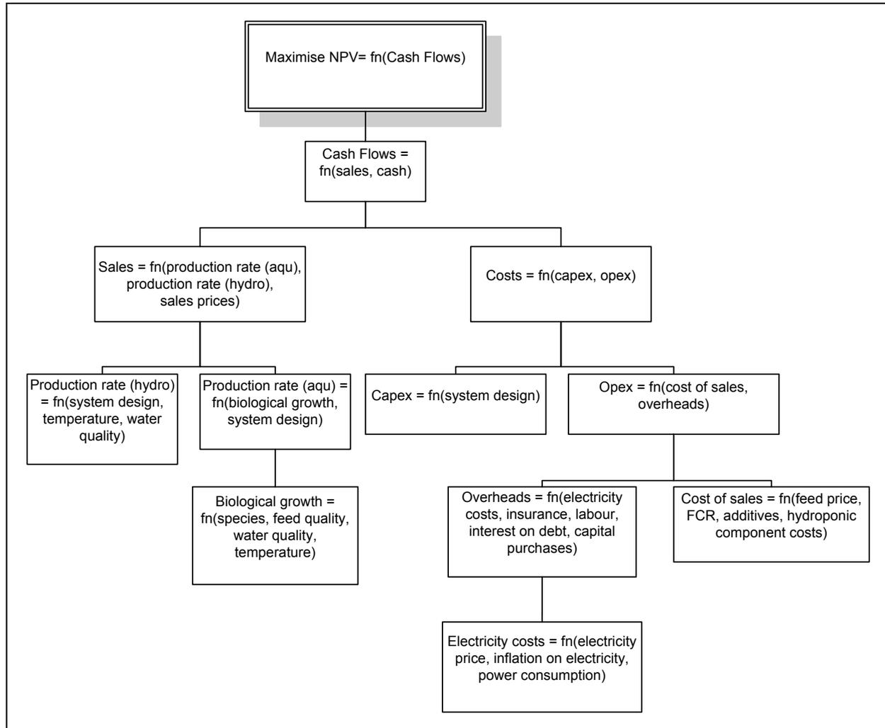
Figure 62 Chart of the entities and parameters that affect the objective function of the near-ideal system
