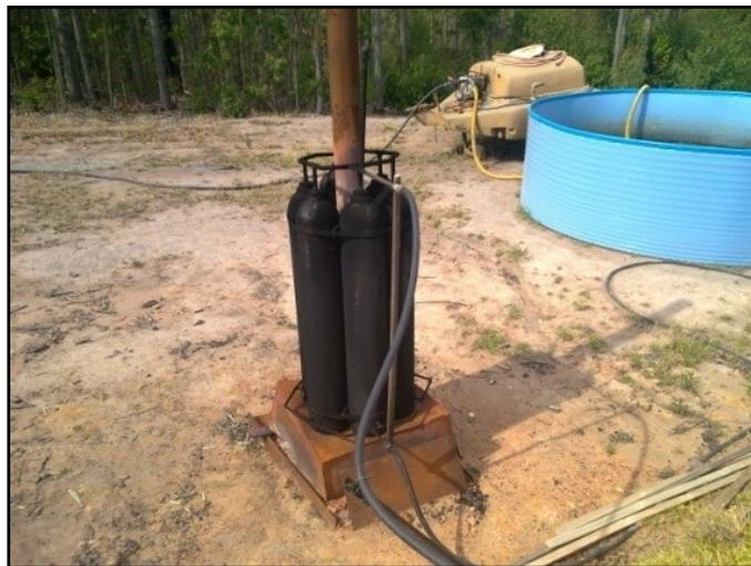
**Figure 21 Wood-fire powered boiler used for heating system water on farm 1**
