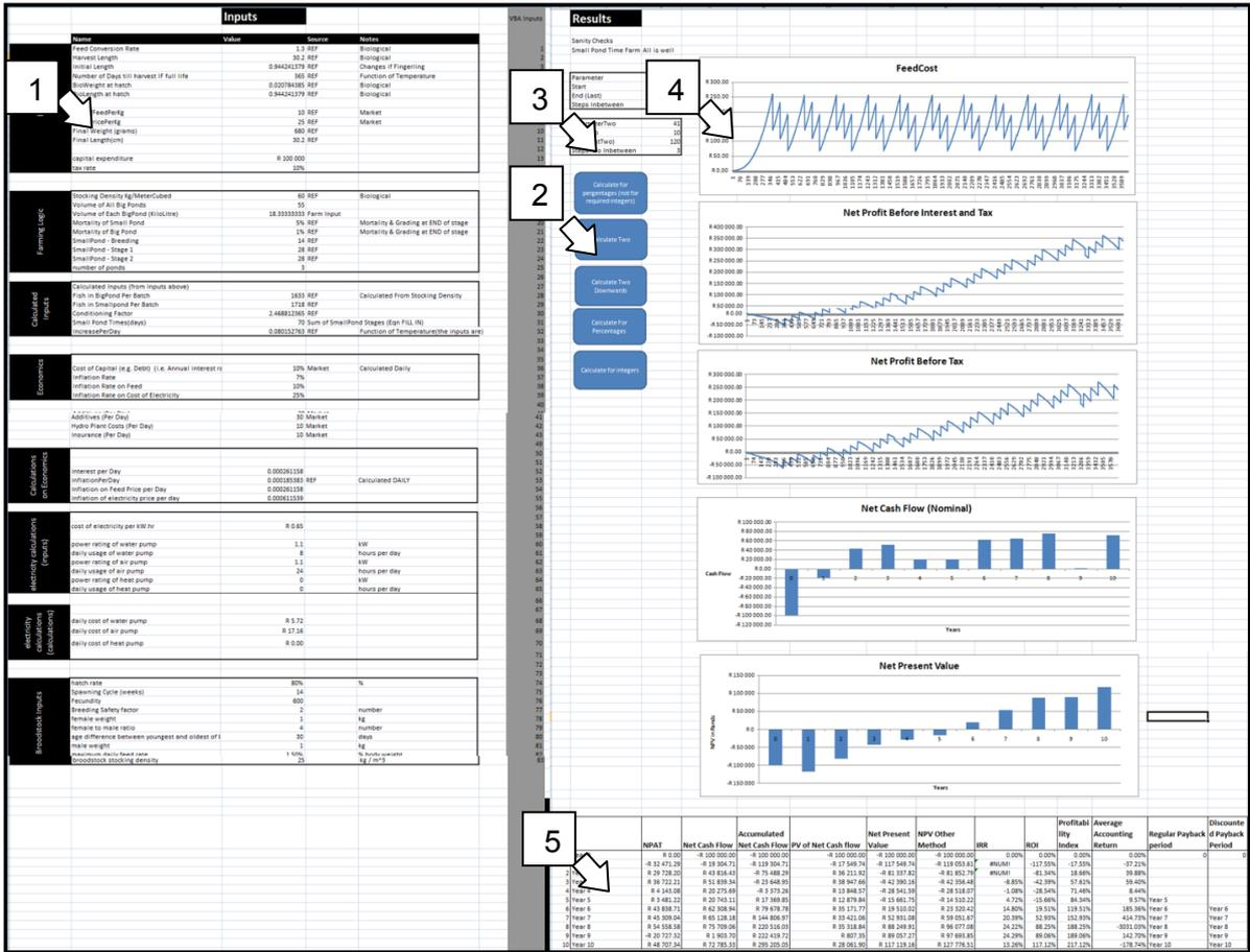
Figure 10 The input sheet of the model, showing input data (1), VBA buttons (2), input cells for the VBA calculations (3), graphs for assistance when testing input parameters (4), and a table showing the performance indicators for the system over a ten-year period (5)
