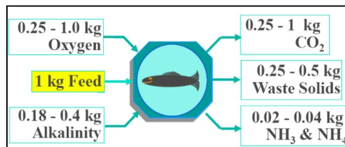
Figure 13 The relation between feed rate and design parameters (Timmons, Clark 2009)
