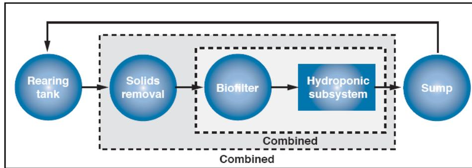
**Figure 8 A typical arrangement of aquaponics system components (Rakocy, Masser & Losordo 2006)**
