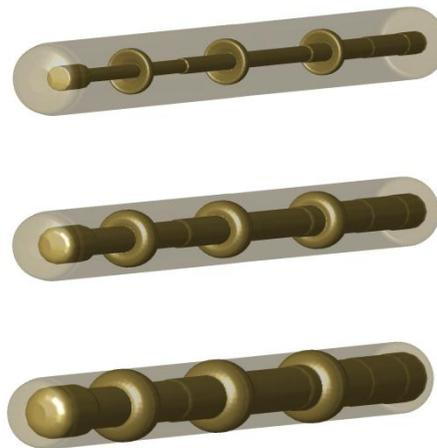
Figure 14: Novel Grain design at various stages of the motor operational phase.
