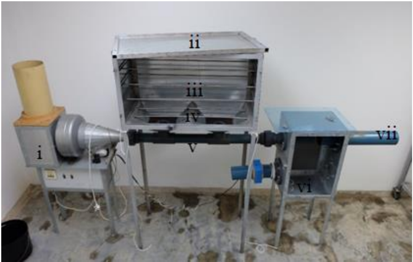
Figure 2.1: Photograph of the assembled collection box. The adult emergence box (iii) lid (ii) is open to display the racks (iii) on which trays containing pupa are placed as well as two vertical square stainless steel funnels (iv) leading into the transporting pipe below (v) which has an airstream (10 m/s) supplied by the axial flow induction fan (i). The airstream flows through a plenum box system (vi) which halts airflow where moths exit via the exit pipe (vii)
