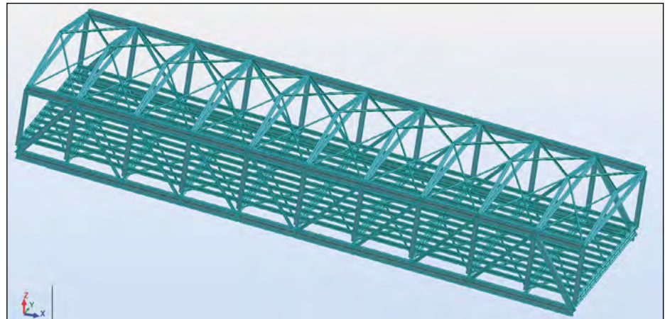
Figure 4 Isometric view of typical steel gantry
