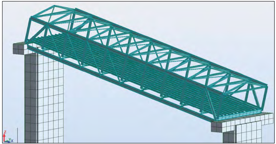
Figure 10 Detail from FE model with shells and 3D gantries
