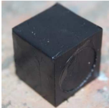
Figure 4-6 - Typical PVC block used in physical laboratory model
