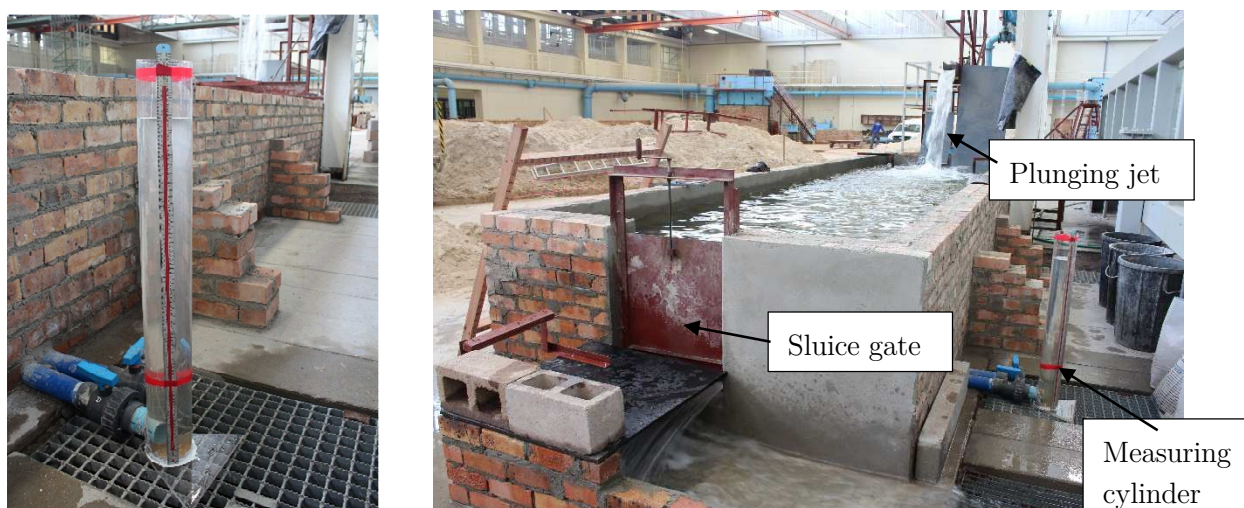
Figure 4-9 - Tailwater measuring cylinder (left) and sluice gate (right)
