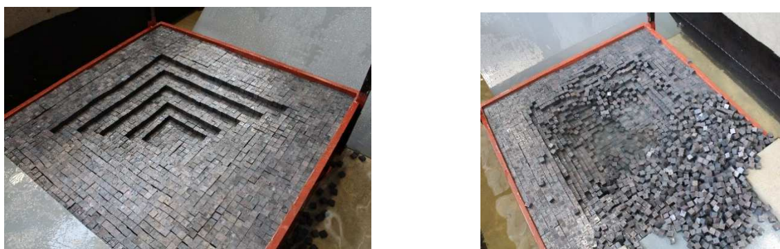
Figure 4-24 - Scour profile using predefined scour hole shape for the 2m drop height including 0.5m tailwater
