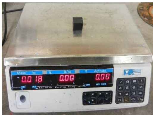
Figure 4-7 - Weight of PVC blocks
