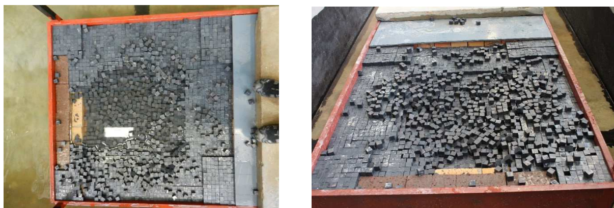
Figure 4-17 - Scour profile for the 4m drop height with a 0.5m tailwater
