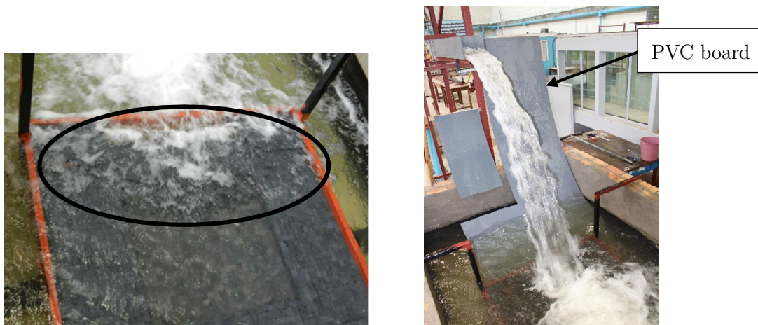
Figure 4-14 - Premature scouring due to large flow during the filling of the plunge pool (left) and PVC board used to control flow (right)
