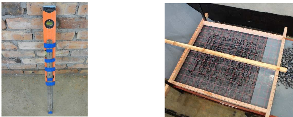
Figure 4-15 - Scour hole depth measuring instrument (left) and measuring grid (right)
