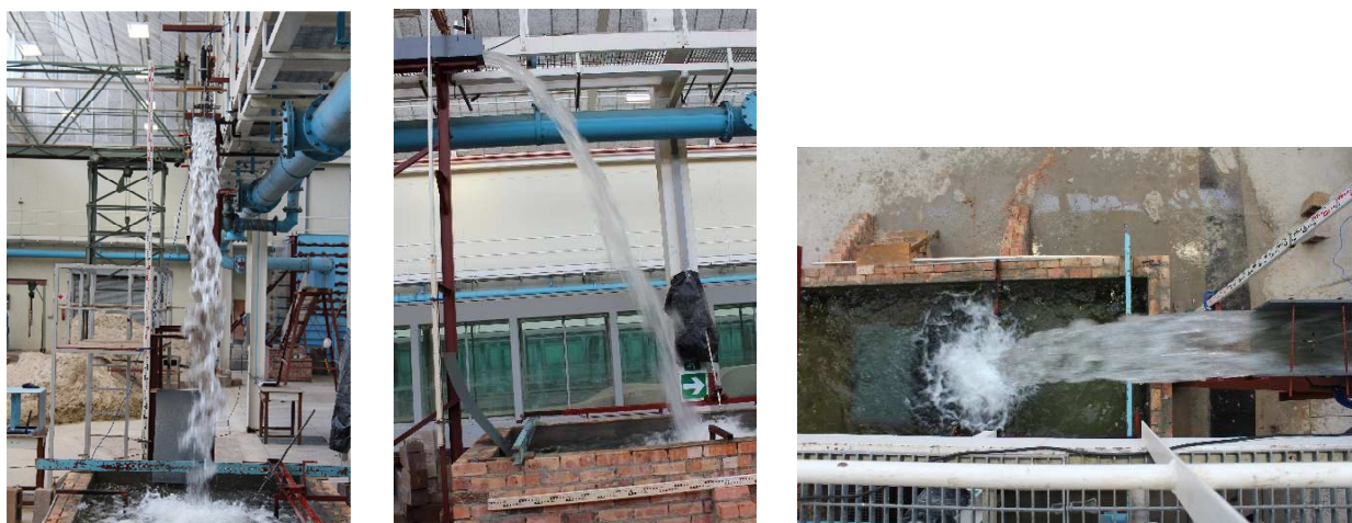
Figure 4-13 - 20l/s discharge and 4m drop height including 0.5m tailwater. Lateral jet profile (left), longitudinal jet profile (middle) and plan view of jet (right)
