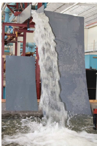
Figure 4-23 - Jet impact conditions for 2m drop height including 0.5m tailwater
