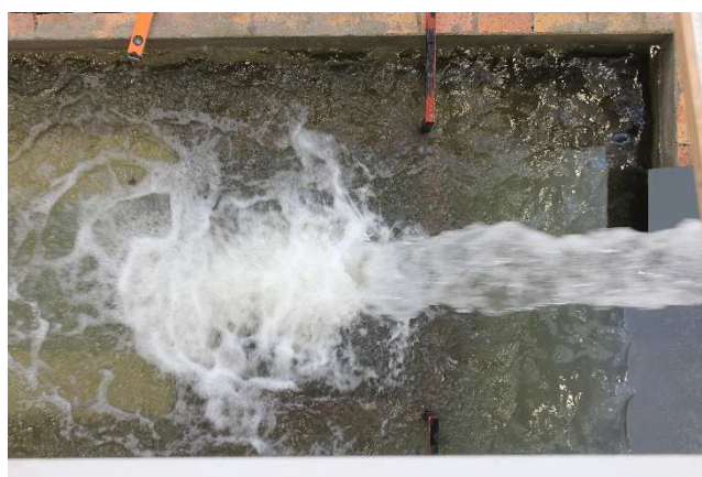
Figure 4-23 - Jet impact conditions for 2m drop height including 0.5m tailwater
