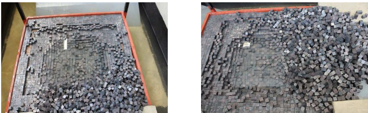
Figure 4-25 - Scour profile for the 2m drop height with 0.5m tailwater
