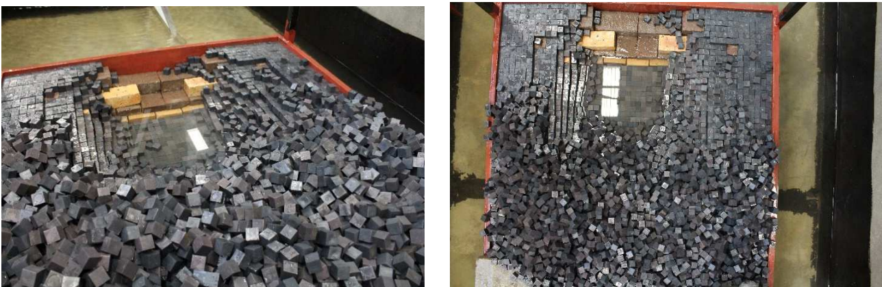
Figure 4-20 - Scour profile for the 3m drop height with 0.5m tailwater
