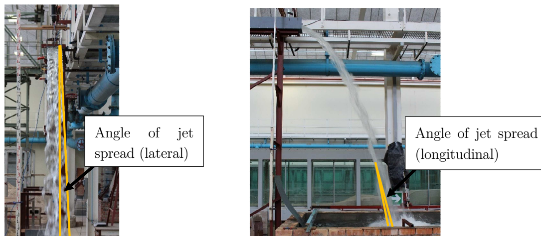
Figure 4-12 - Lateral (left) and longitudinal (right) spreading angle of the jet
