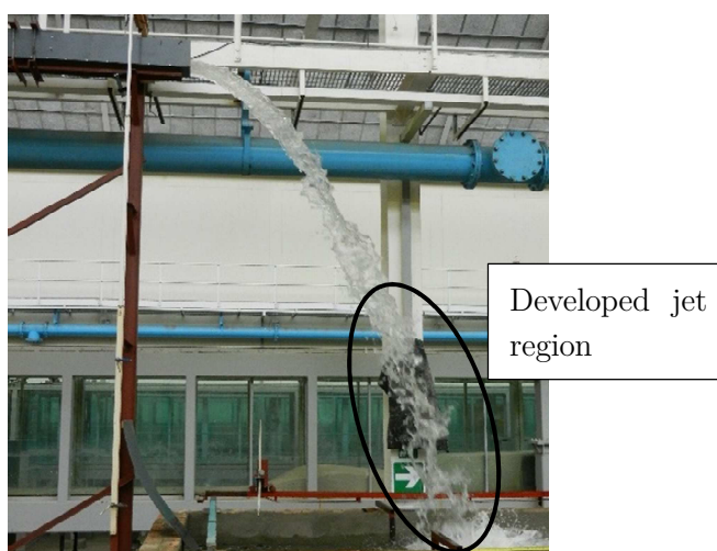
Figure 4-18 - Developed jet at impact for 4m drop height including 0.5m tailwater (physical laboratory model)
