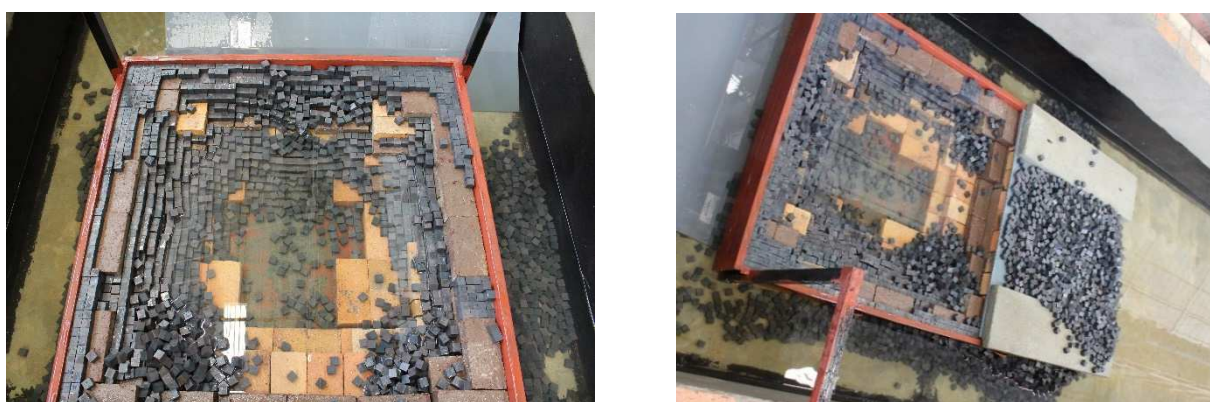
Figure 4-26 - Scour profile for the 2m drop height with 0.25m tailwater
