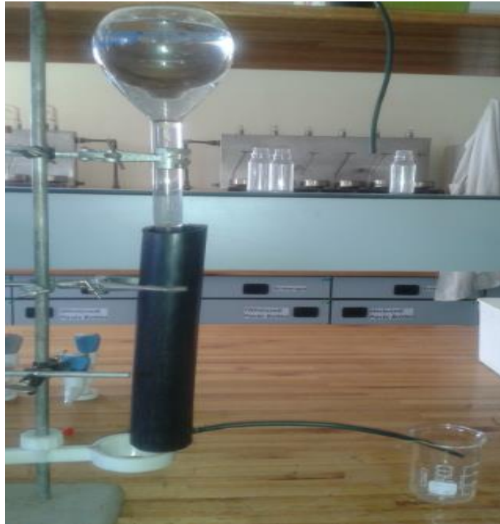
Figure 3.1. Column experimental setup showing the inverted volumetric flask maintained at constant pressure head and the effluent pipe inserted into the collecting flask
