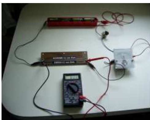
Figure 4.8 Experimental set up to determine Ohm's law
