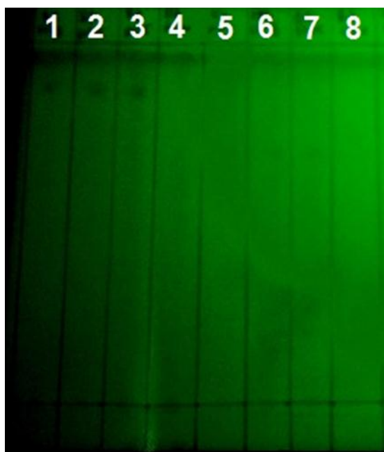
Figure K1: Developed TLC visualised under short wave 254 nm ultraviolet light. Benzene extracts separated using a solvent system consisting of chloroform: formic acid: ethyl acetate: n-hexane (5:4:1:0.02 v/v/v/v). Lane 1: pH 3, Lane 2: pH 4, Lane 3: pH 5, Lane 4: pH 6, Lane 5: pH 7, Lane 6: pH 8, Lane 7: pH 9, Lane 8: Benzene solvent control.
