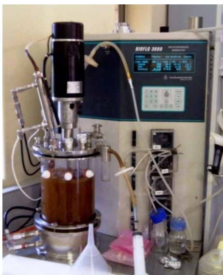
Figure 3.11: BIOFLO 3000 Continuous Stirred Tank Reactor.
