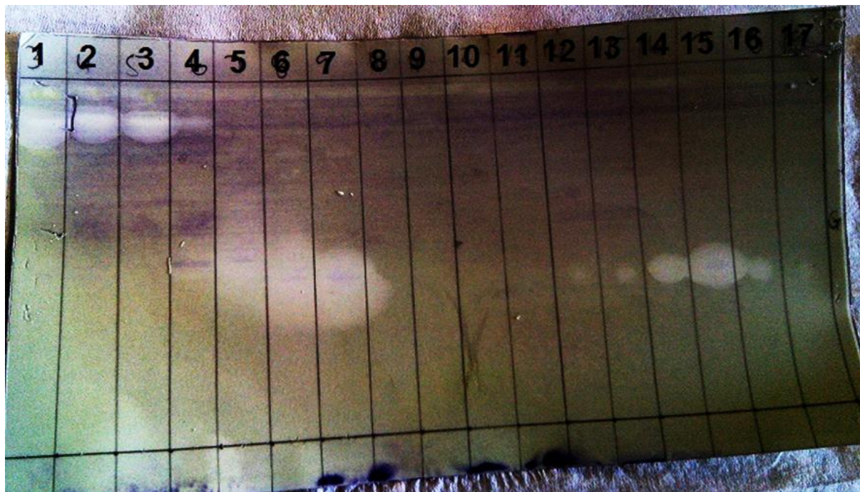
Figure L1: Bioautography assay of silica gel purified crude EtOAc extracts from airlift reactor fermentation broth against DRW isolate S. aureus 4. Lane 1 – 17: Fractions 1 – 17.
