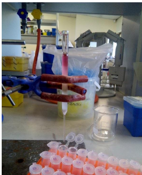
Figure 5.4: 4.5 mm diameter glass Pasteur pipette containing 10 % v/v water deactivated silica. Compounds were eluted with a gradient elution method.
