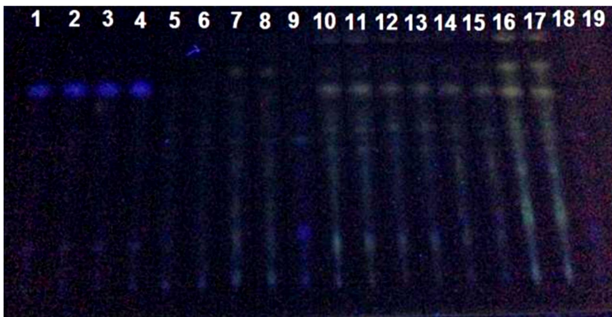
Figure D4: Developed TLC visualised under long wave 365 nm ultraviolet light. Ethyl acetate extracts separated using a solvent system consisting of chloroform: formic acid: ethyl acetate: n-hexane (5:4:1:0.02 v/v/v/v). Testing the effects of scale-up from 1 litre to 2 litre baffled flasks on antimicrobial production by S. pharetrae sp. strain CZA14 T cultured in 153 + glycerol, pH 6.0, 30 °C at 160 rpm for 3 – 10 days.. Lane 1 and 2: EtOAc extracts – from supernatant filtrate (SNF), day 3 in duplicate. Lanes 3 and 4: EtOAc extracts – from SNF, day 5 in duplicate. Lanes 5 and 6: EtOAc extracts – from SNF, day 7 in duplicate. Lanes 7 and 8: EtOAc extracts – from SNF, day 10 in duplicate. Lane 9: 153 + glycerol, pH 6.0 media control. Lanes 10 and 11: EtOAc extracts – from cell mass (cell), day 3 in duplicate. Lanes 12 and 13: EtOAc extracts – from cell, day 5 in duplicate. Lanes 14 and 15: EtOAc extracts – from cell, day 7 in duplicate. Lanes 16 and 17: EtOAc extracts – from cell, day 10 in duplicate. Lane 18: 153 + glycerol, pH 6.0 media control. Lane 19: EtOAc control.
