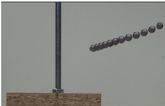
(a) Camera output of mass position
