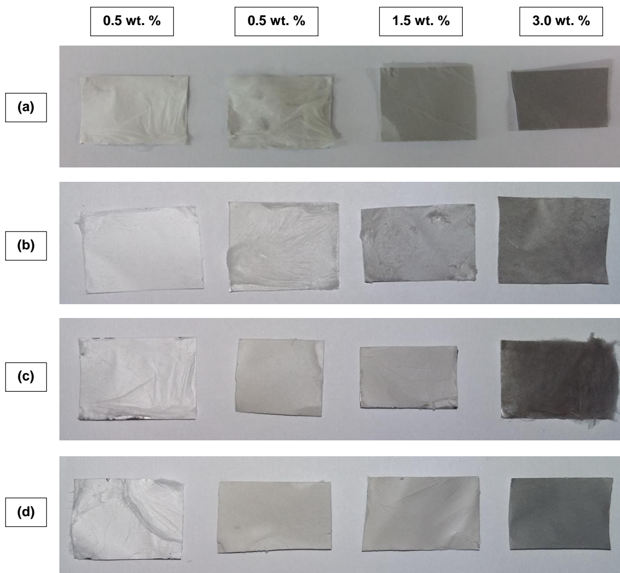
Figure 4.36: Nanofibrous mat of electrospun nanofibres incorporated with (a) MWCNT-PMMA, (b) magnetic CNT-PMMA, (c) ex-situ MWCNT-Fe 3 O 4 and (d) in-situ MWCNT-Fe 3 O 4 .
