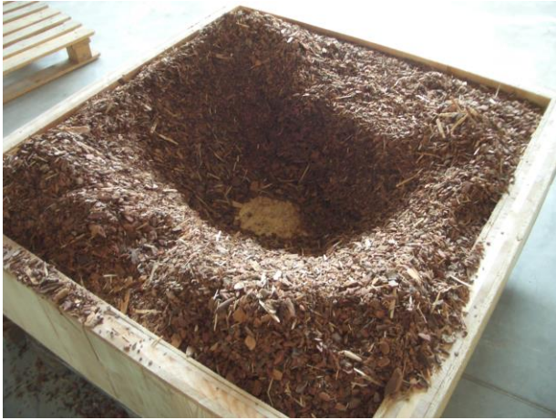
Fig. 1. Bark fill material for the wall construction (particle size 8–30 mm)
