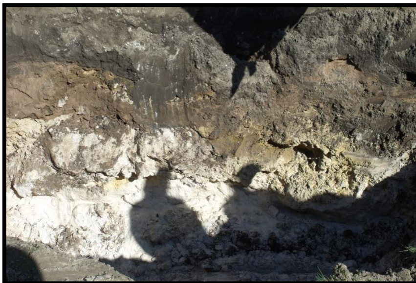
Figure 39: The top dark grey brown sand, while the bottom section of the soil displays a calcareous sand and clay type soil. The area that is smeared just above the calcareous layers marks the depth to water table
