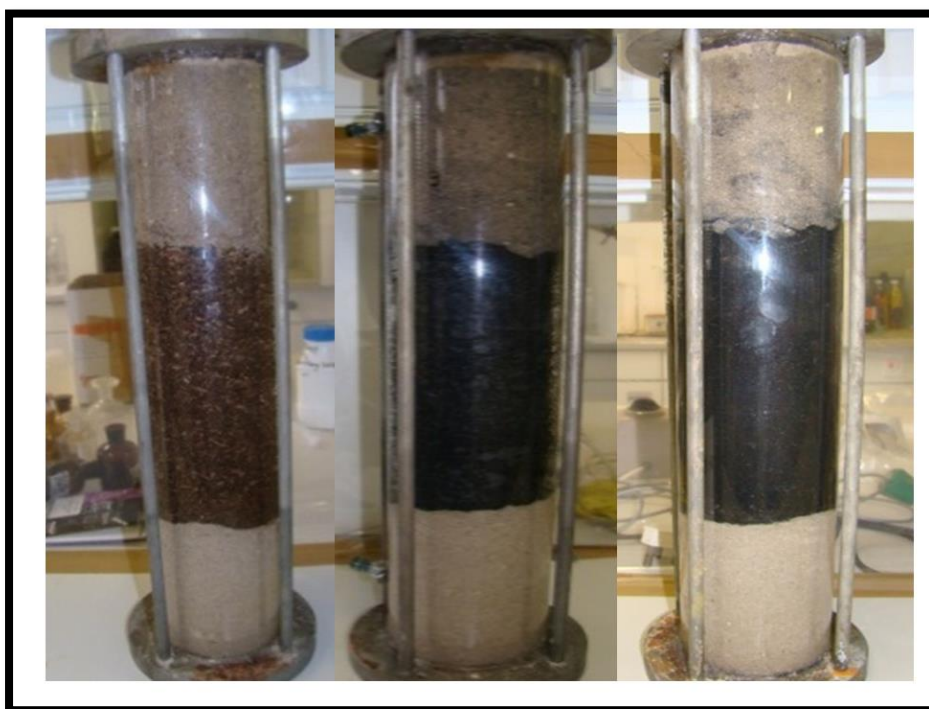
Figure 7: Pictures of columns packed with sand, woodchips (35 month) (left), woodchips (27 month) and biochar (middle) and biochar only (right)
