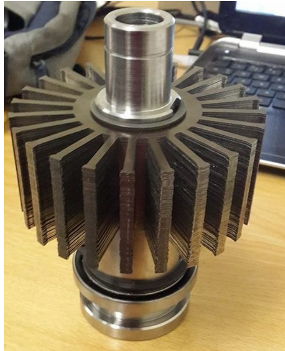
(b) Stator core.
