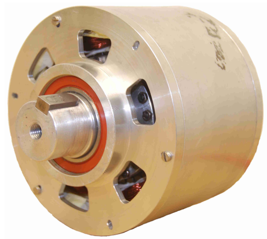
(b) Ring-stator MGM
