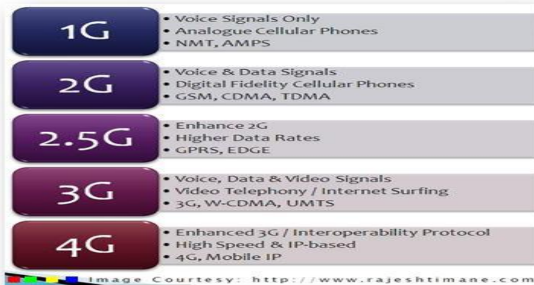
Figure 3.5 The key data features of 1G, 2G, 2.5G, 3G, and 4G mobile phones
