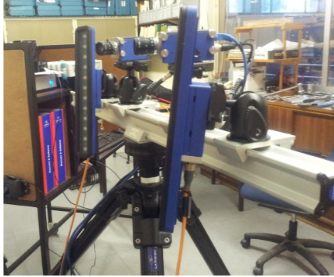
Figure A.3: Digital image correlation camera set up
