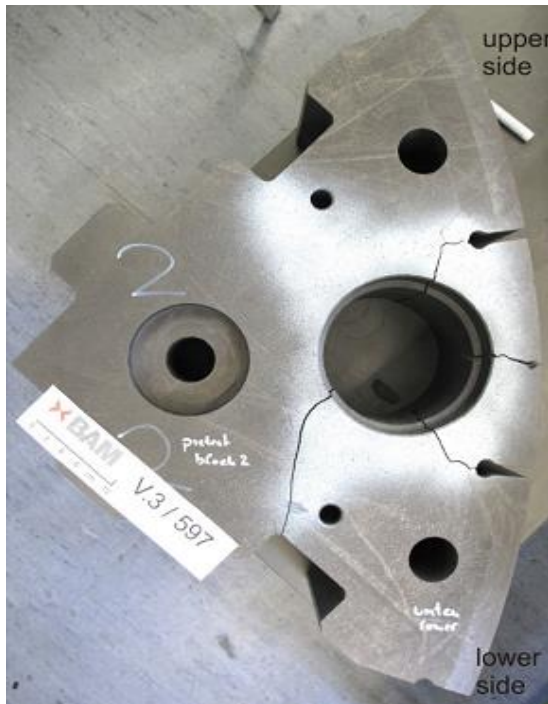
Figure 9-8: Actual failure locations [127]
