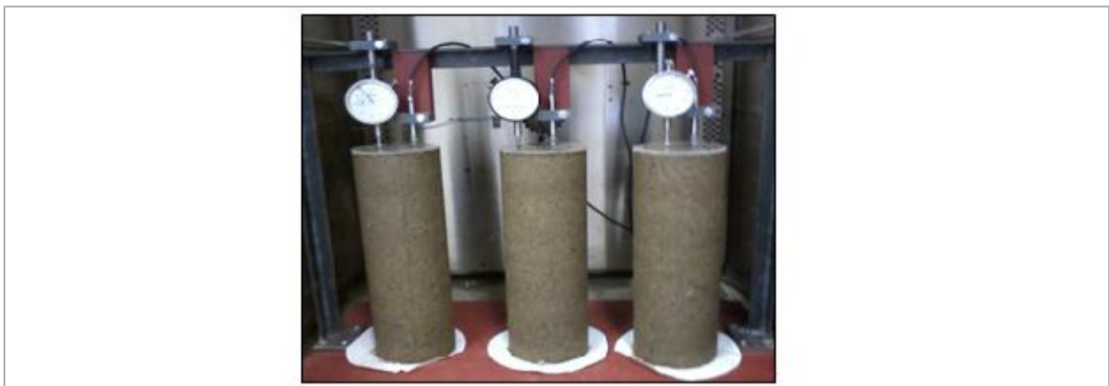
Figure 5.8 Rigid frame used for testing three cylindrical specimens simultaneously.
