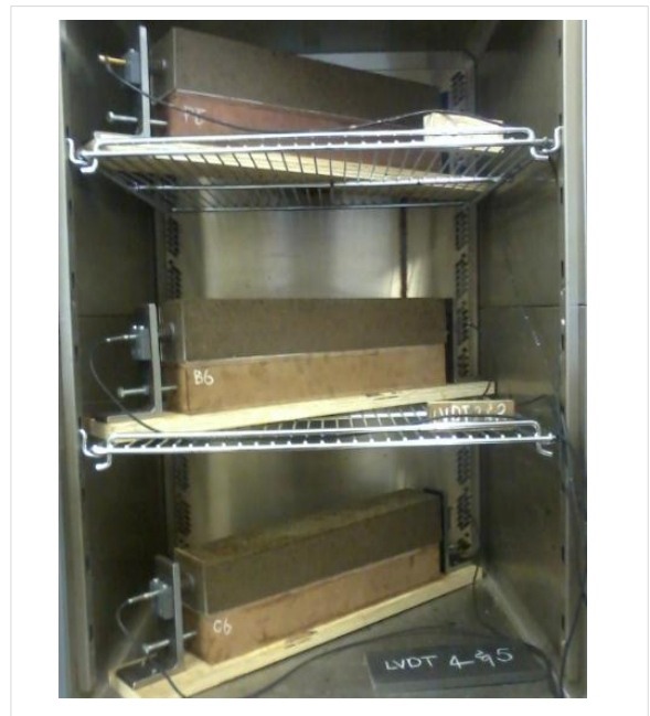
Figure 5.7 Three rigid frames used to test three beam specimens simultaneously.
