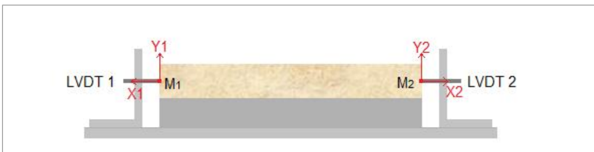
Figure 6.1 LVDT placement during beam shrinkage testing.
