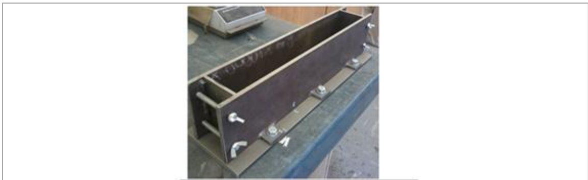
Figure 5.3 Beam split mould, designed for fast and easy specimen removal.
