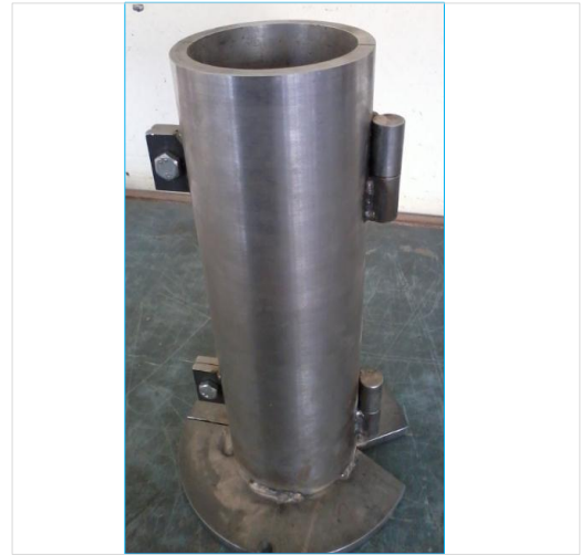
Figure 5.5 Cylindrical split mould, designed for fast and easy specimen removal.
