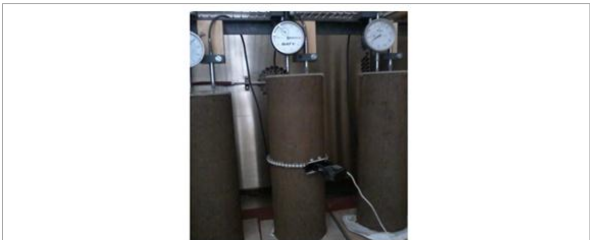
Figure 5.9 Placement of cylindrical LVDT on cylindrical specimen.
