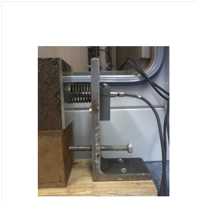
Figure 5.6 Positioning of Perspex squares and LVDTs before testing.
