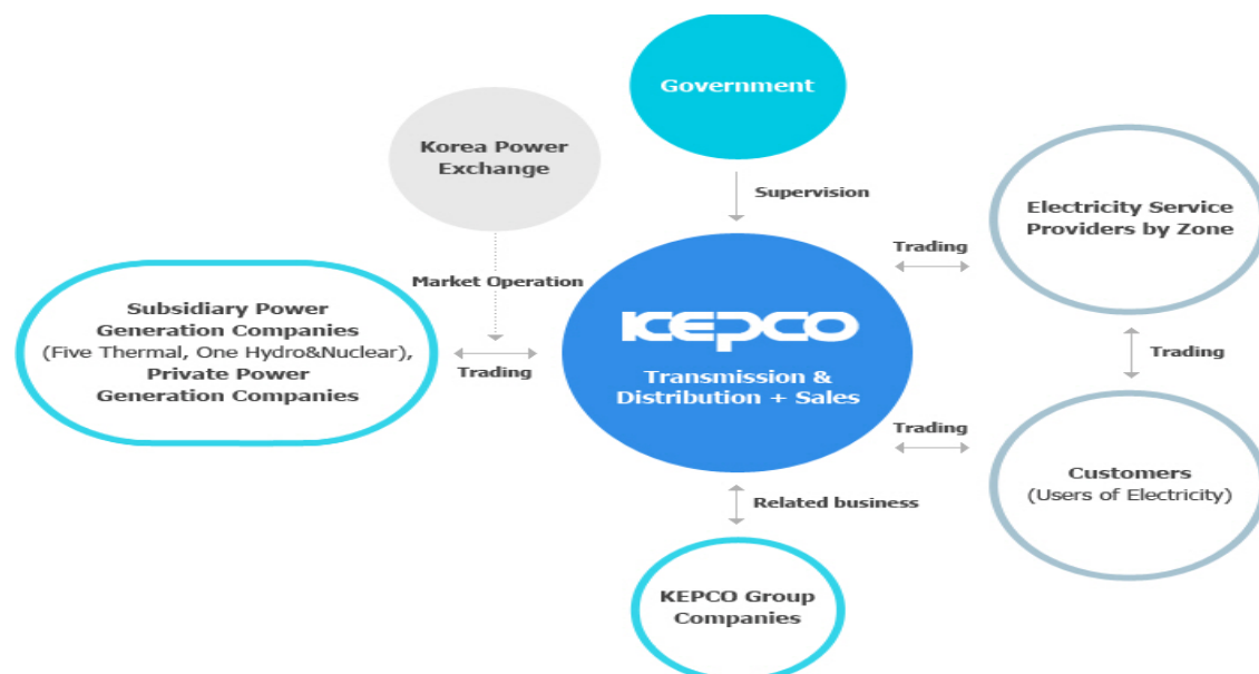
Figure 4.9 Structure of South Korea's electricity industry
