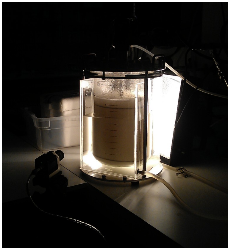
Figure E.2: Initial Lighting Configuration for Recording the Interfacial Area
