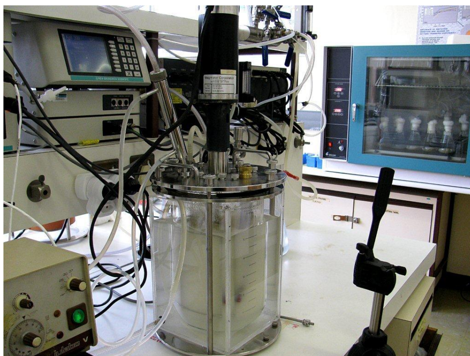
Figure 4.7: Bioreactor and Water Jacket in Operation
