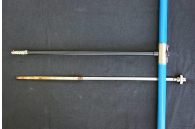
Figure 2: Haglof increment borer with extractor tray and core sample
