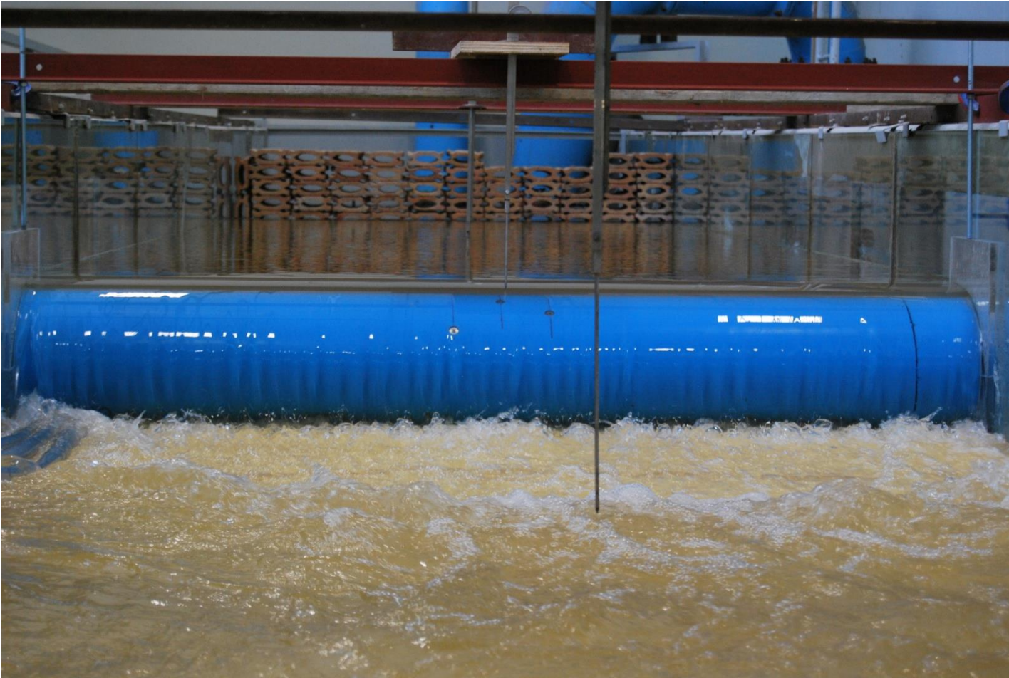
Hydraulic jump at 41.208l/s over a 0.25m diameter weir
