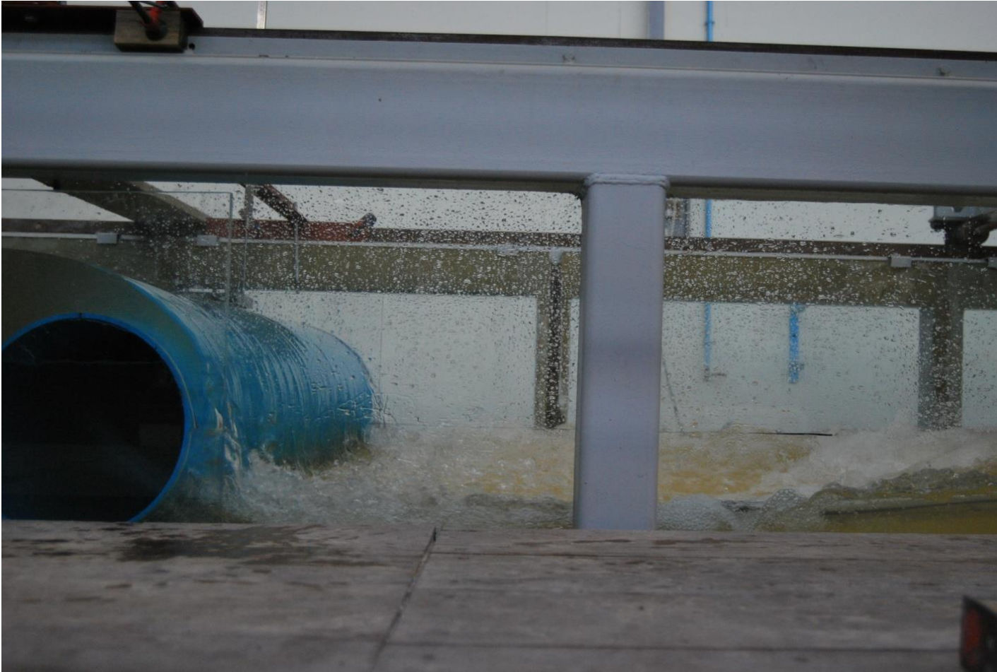
Hydraulic jump at 98.709l/s over a 0.3m diameter weir
