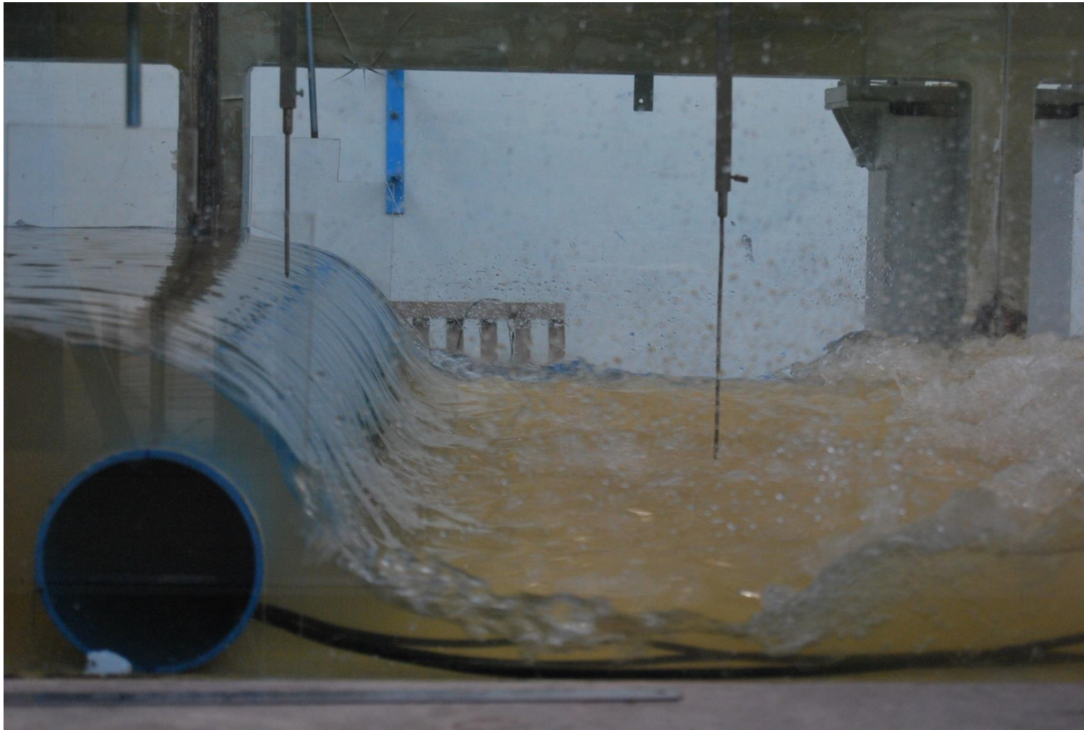
Hydraulic jump at 101.9l/s over a 0.1m diameter weir
