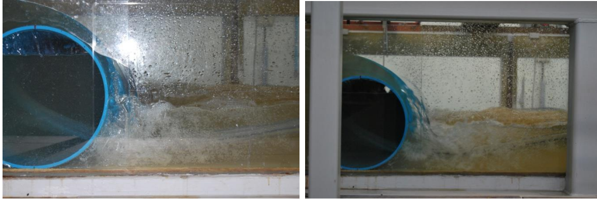
Figure 3.6 Submerged jumps at 53.028 l/s (left) and 143.43 l/s (right) (viewed from US laboratory)
