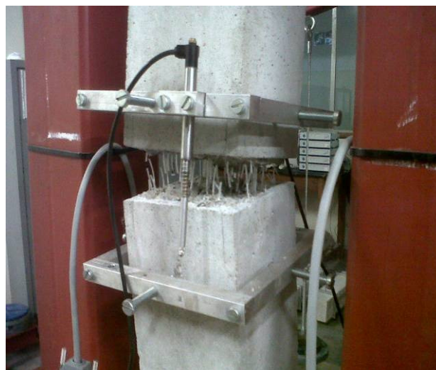
Figure 5.14: Tensile creep failure of specimen showing pulled out fibres
