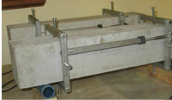
Figure 3.9: Shrinkage test specimens showing frame with LVDT extenders
