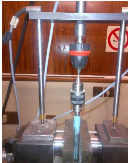
Figure 3.14: Single fibre tensile strength test
