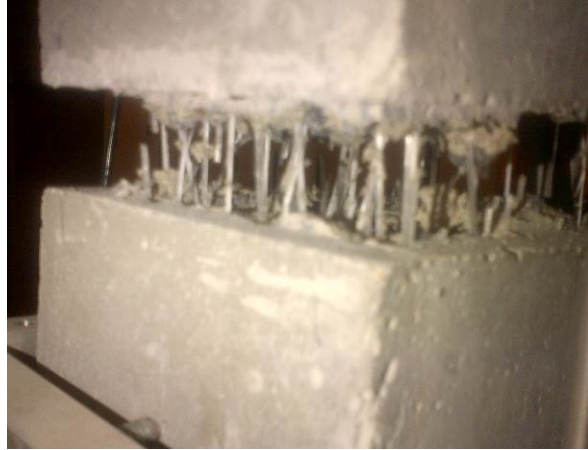
Figure 4.3: Fibre aligned in the direction of loading
