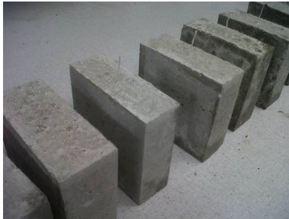
Figure 3.12: Single fibre pullout test specimens
