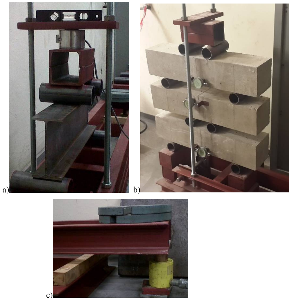
Figure 3.18: Flexural creep setup (a) Calibration of frame showing load cell (b) Constant load and Enerpac cylinder (c) Stacked beams already loaded
