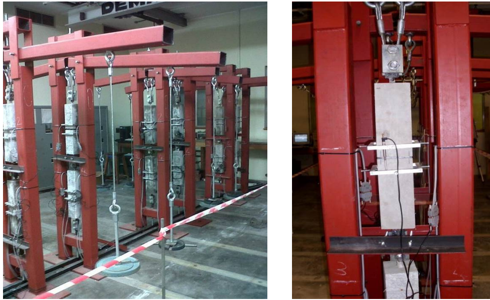
Figure 3.8: Creep frames showing specimens under sustained loads and LVDT position over a gauge length of 70 mm.
