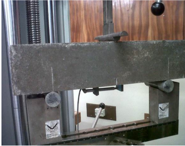
Figure 3.16: Flexural tensile test under three point loading
