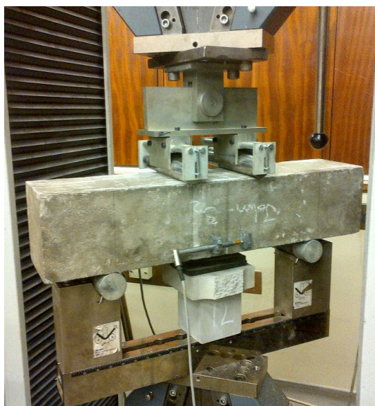
Figure 3.17: Flexural tensile test under four point loading
