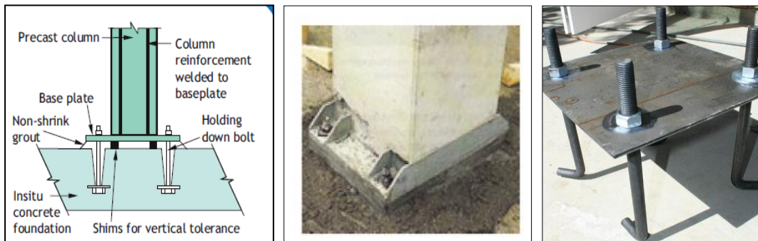
Figure 6.7 - Illustration of the baseplate connection type (The Shockey Precast Group 2001)
