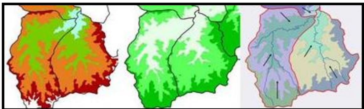
Figure 4.4: Sub-delineation of quaternary catchments from altitude (left) into three quinary catchments by natural breaks (middle) with flow paths (right) of water Source: Schulze and Horan (2010)
