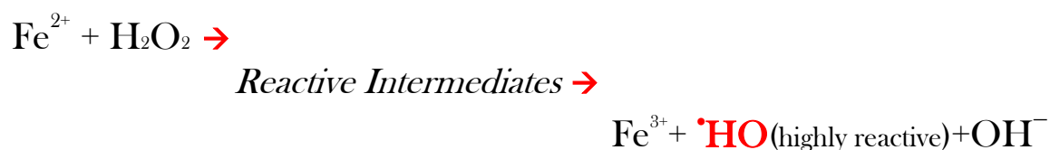
Figure 2 Formation of active ROS by "Fenton-type" reaction
