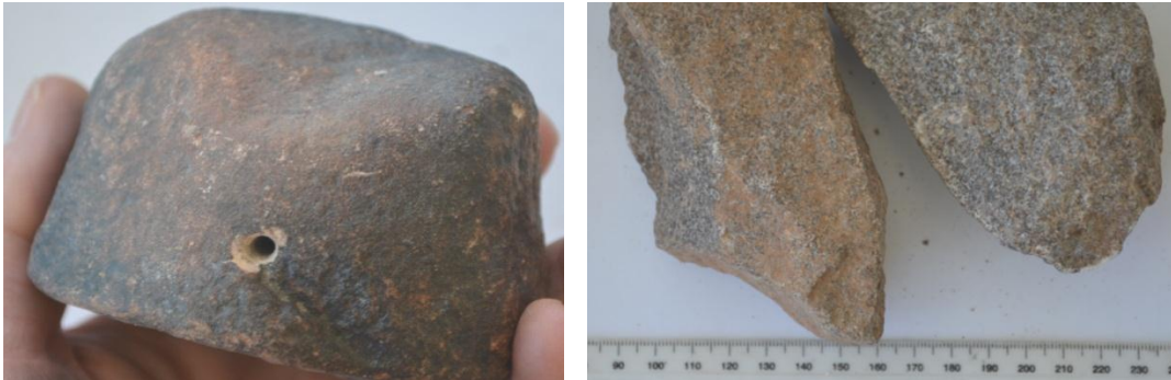
Figure 10: Dolerite: a loose sample from the ground; crushed samples (1500 cycles)
