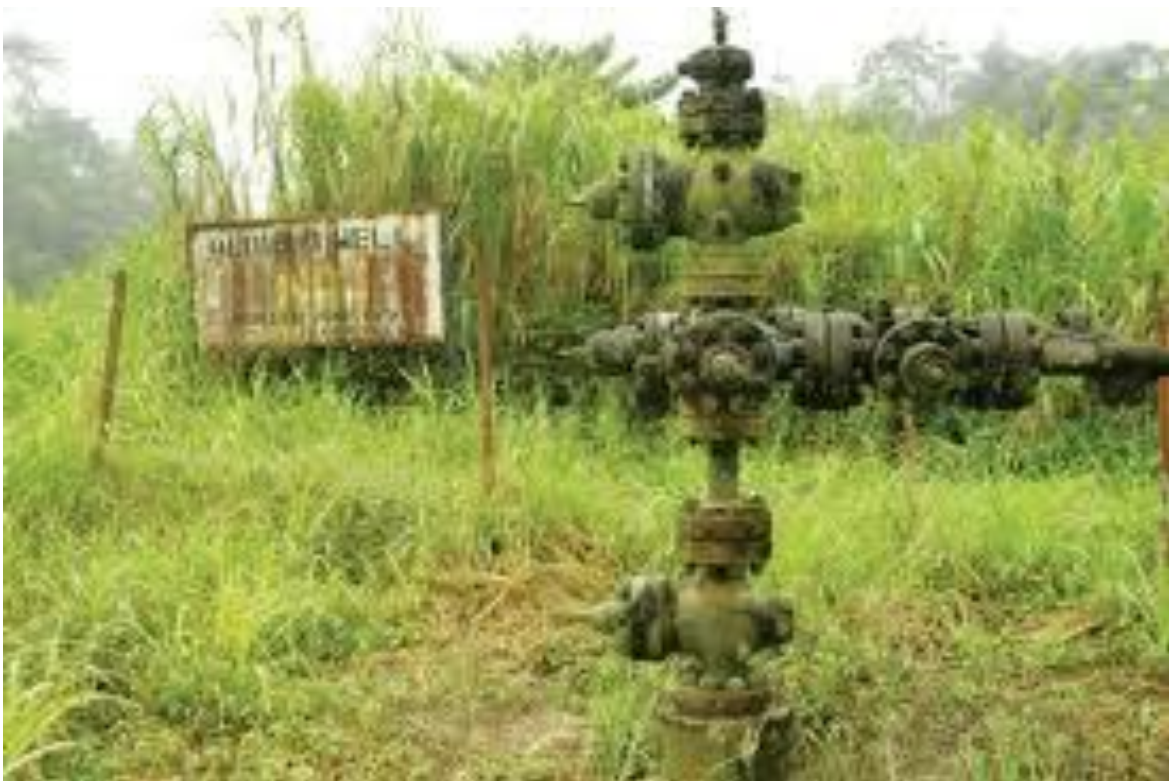
Plate 1 a : A relatively more detailed photograph of the first oil-well. It captures more clearly the site of the first find of oil showing the first wellhead: it is also known as “Christmas Tree”. On the timeworn, rusted sign is written “Oloibiri Well No. 1. Drilled June, 1956. Depth: 12, 000 Feet”. These photographs are viral images on Google whose source cannot be established.
