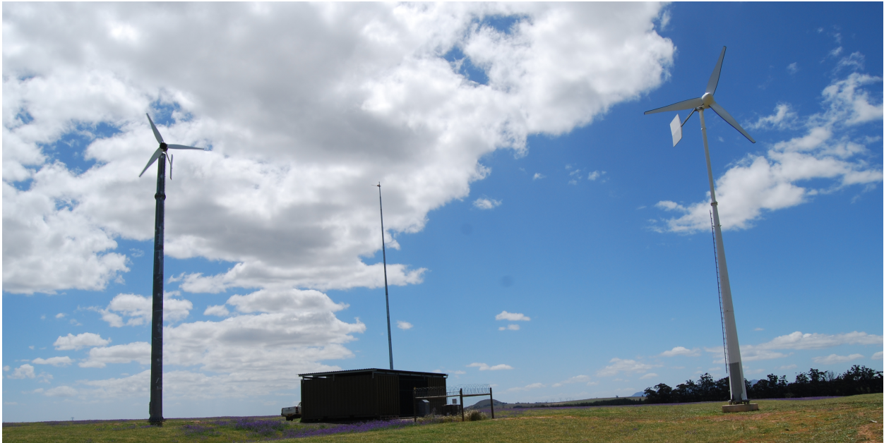
Figure 7.30: SS-PMG 1 and SS-PMG 2 being field tested at the Stellenbosch University Mariendahl small wind turbine field testing facility.
