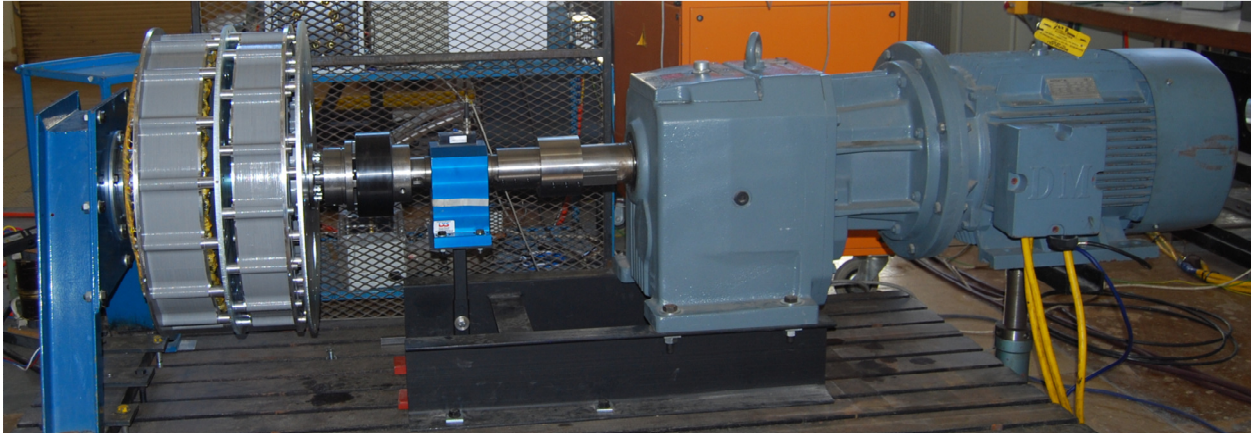
Figure 7.2: Prototype 15 kW SS-PMG 2 on the testbench connected to a driving motor on the left through a torque sensor shown in the middle.
