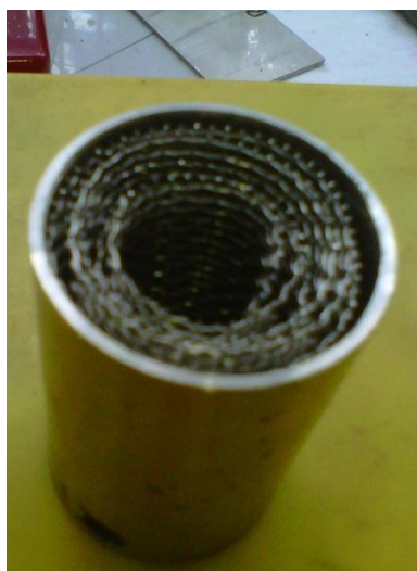
Figure 17: Mesh Wire Water Trap
