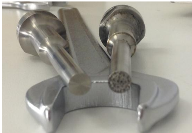
Figure 49: Ultrasonic Probe tip damage after experiments were conducted
