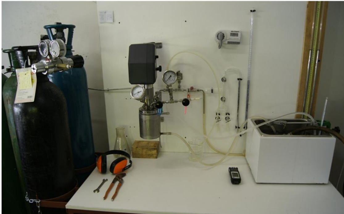
Figure 13: Experimental Setup for partial oxidation of bacterial sludge using ultrasound
