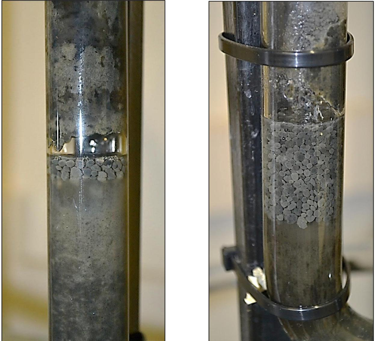
**Figure 6** Images of granule washout in the U-tubes of  $R_{\text{ozone}}$  (left) and  $R_{\text{control}}$  (right).
