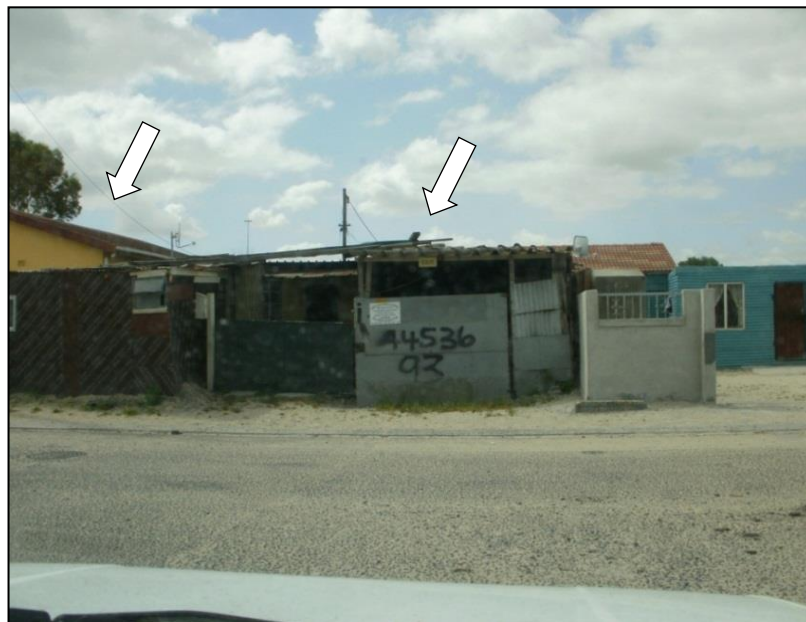
Figure 6.3. Illegal and informal extensions to an original house provided through the upgrading process in Makhaza, Cape Town. The arrows indicate the original house (Massey 2011)
